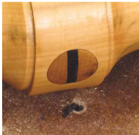
▲ Pic.35 After the end is carefully sanded you can see how effective the ebony looks against the boxwood. The handle is finished with food-safe oil just like the bowl
